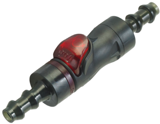
Everis™ PLQ2 Nominal flow of 1/8" (3.2 mm) with a Cv of 0.37 (Kv 0.32) Termination options: Locking hose barb, SAE, G thread
